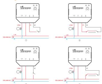
① For the above ③④ wiring methods, please ensure the proper wiring and powering of the L in terminal, otherwise it will cause the device to work abnormally.
